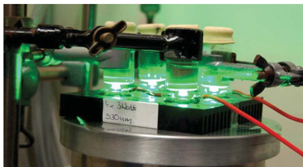
Fig. 1 Reaction vials irradiated by an array of high power green light LEDs.
